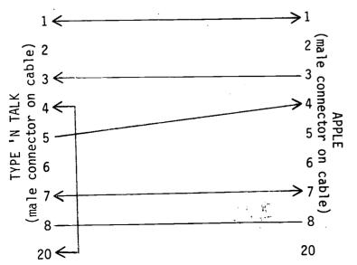
\*\*First choice because of handshaking and output to the computer's CRT \*Second choice - handshaking, but no output to computer's CRT
