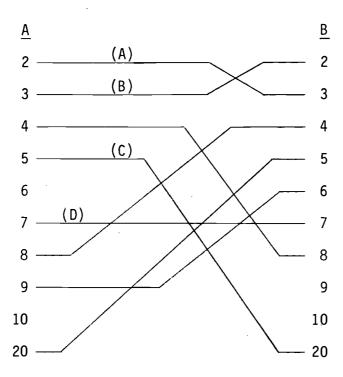
NOTES: To use VersaBraille model P2C with PCBRAILLE, only wires (A), (B), and (D) are required. A 25 pin FEMALE "D" connector is needed on both ends of the cable.
