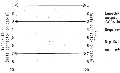
Lengthy transmissions will cause some output to be skipped when synthesizer falls behind. (No handshaking)
