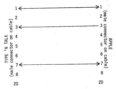
Lengthy transmissions will cause some output to be skipped when synthesizer falls behing. (No handshaking)
