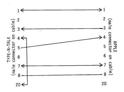
Hardware handshaking prevents loss of output during lengthy transmissions.
