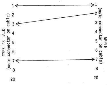
Lengthy transmissions will cause some output to be skipped when synthesizer falls behind. (No handshaking)
