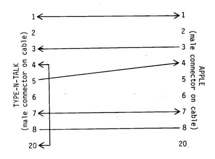
Version A - Hardware handshaking prevents loss of output during lengthy transmissions. Computer's CRT will be disconnected when the TYPE-N-TALK is initialized.
