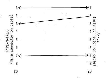
Lengthy transmissions will cause some output to be skipped when synthesizer falls behind. (No handshaking)
